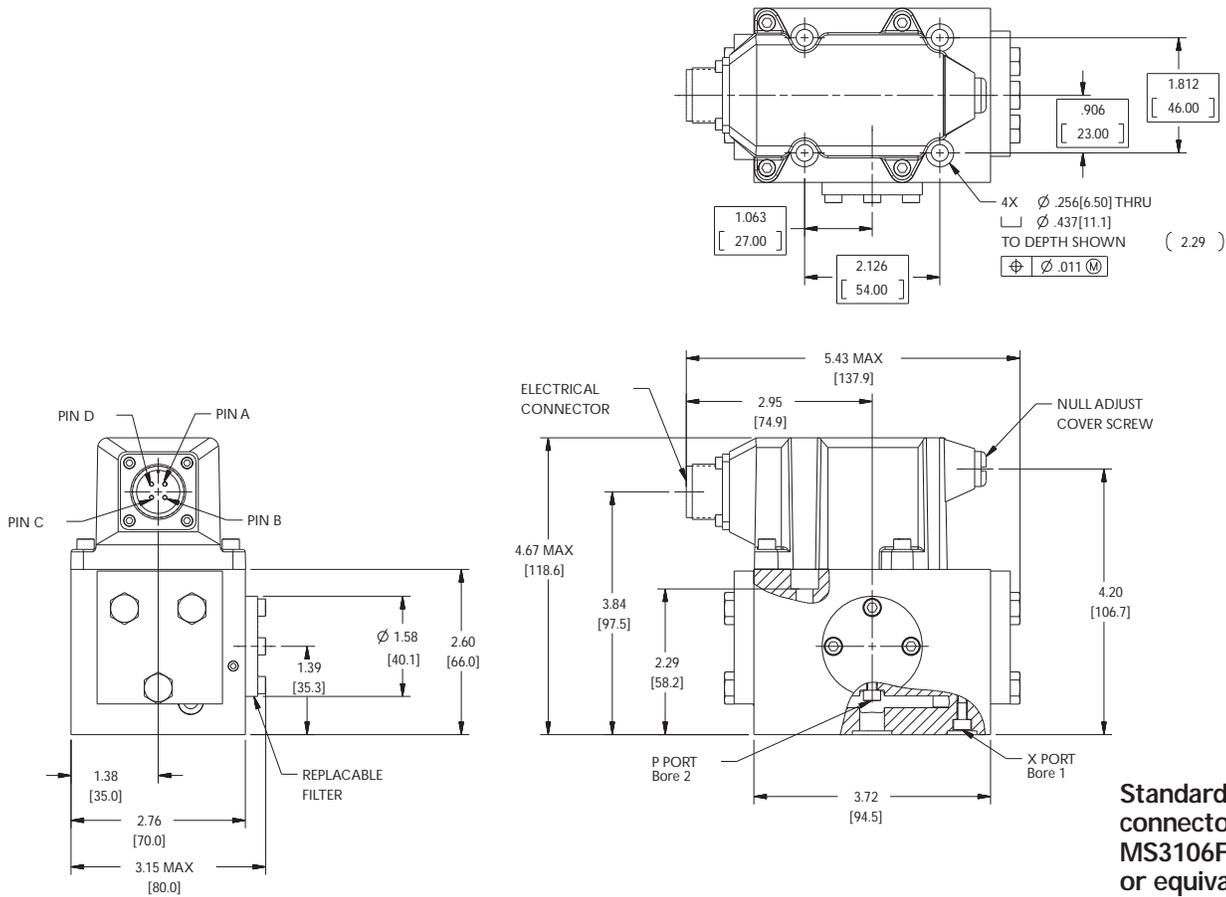
Standard electrical connector mates with MS3106F14S-2S or equivalent.
